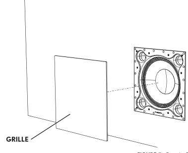
**FIGURE 1b.** Once the Grille Frame has been installed, carefully cap the Grille over the Frame.
