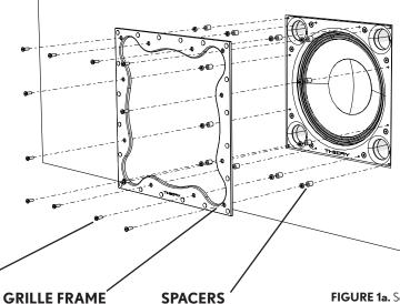
FIGURE 1a. Secure the plastic Grille Frame to the Speaker Assembly baffle using the socket flange-head screws and spacers supplied with the grille kit.
